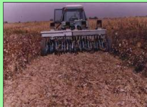
Figure 2. Complex aggregate KM-3, which combines soil tillage, sowing of wheat in the inter-rows of cotton, applying of fertilizers, chopping stems and making furrows.
