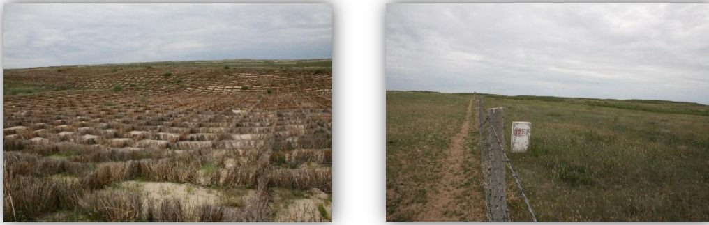
Figure 2-13. The mechanical sand barrier inside the enclosed area and vegetation growth in comparison with the outside in August 2017
