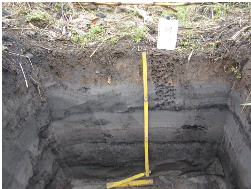
FIGURE 16. Indirect recultivation – covering the deposited ash and slag with soil at TP Tuzla (Photo: H. Čustović)
