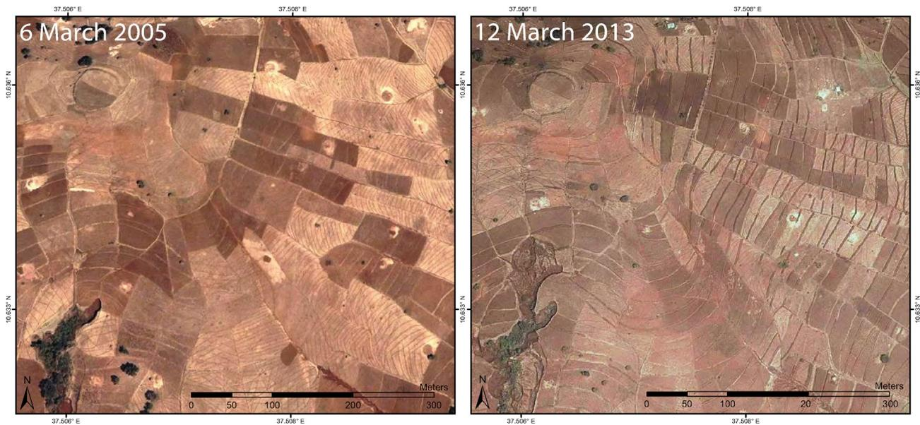
Fig. 3. Google Earth images from the years 2005 and 2013, showing new fanya juu terraces and an increasing gully (bottom left) in the Gerda catchment.
